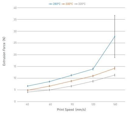
Test parameters: 12mm length brass heat block, BMG extruder, Phaetus Hardened Steel Nozzle, Nozzle size 0.4mm, Layer Height 0.2mm.
